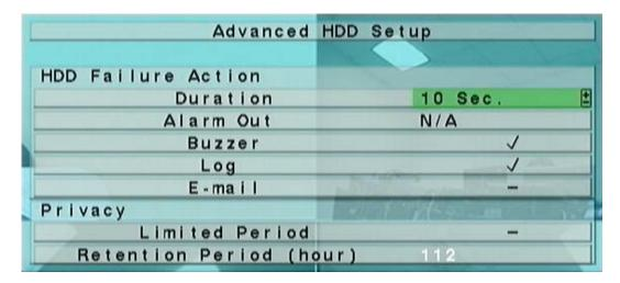
The HDD Failure Action in Advanced HDD Setup allows the administrator to define how the system responds to the detected HDD failure, while the Privacy settings allow the administrator to set the DVR to record for Limited Period and the Retention Period of its HDD storage. The HDD Failure Action will be triggered if there's no available formatted HDD detected.
