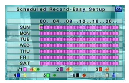
The Scheduled Record – Easy Setup allows the administrator to use a simpler and easier way to setup the scheduled record of the system. In Easy Setup, there are **Six Selectable Recording Modes:** Alarm+Motion+Normal, Alarm+Motion, Alarm,
