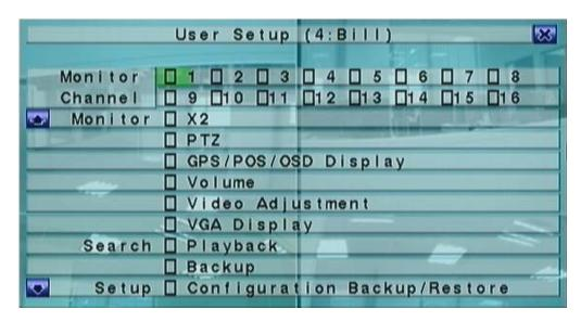
The Advanced User Setup allows the administrator to setup each user's detailed access right of the system.
