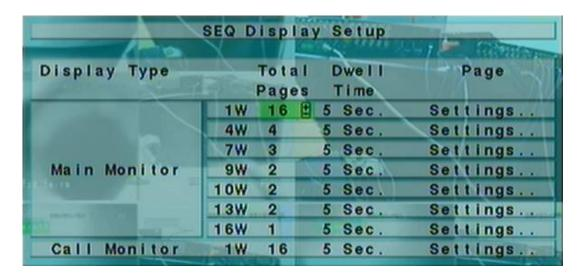
The SEQ Display Setup allows the administrator to define the display pages in SEQ Display for main monitor and call monitor. There are up to 7 display types - 1-Window, 4-Window, 7-Window, 9-Window, 10-Window, 13-Window and 16-Window - for main monitor, and 1 display type for call monitor.
