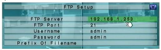
The FTP Setup allows the administrator to set FTP related parameters. When an event occurs and FTP is enabled for the action, the recorded video/audio for that event will be sent to the FTP server based on the parameters set here.
