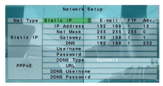
The Network Setup allows the administrator to setup all Ethernet network related parameters. Please check with your network administrator to set these parameters correctly.
