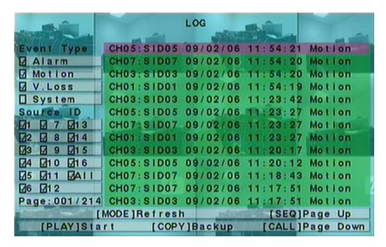
There are four different types of event logs, including Alarm, Motion, Video Loss, and System. And up to 3000 most recent event logs can be stored in the system.
