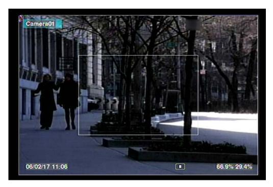
The system supports X2/X4 Digital Zoom function. To use this function, press X2 button (Mouse: ) in full screen display to enter Digital Zoom mode. There will be a zoom window shown in the video window as shown. The zoom window (a) will always be shown at zoom factor X1, (b) can be shown or hidden at zoom factor X2, and (c) will never be shown at zoom factor X4. The operations in Digital Zoom mode are as below:
