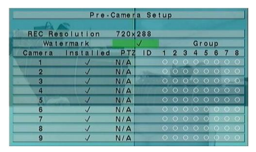
There are up to 16/9 cameras which can be connected to the system. The Pre-Camera Setup allows the administrator to define some fundamental attributes, which may relate one camera to the others, for all the installed cameras.
