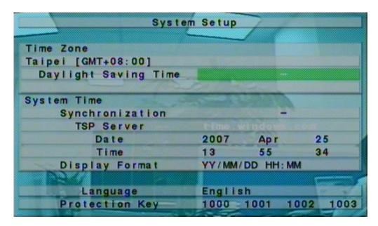
The System Setup allows the administrator to set the system time, time zone, time synchronization, language, etc.
