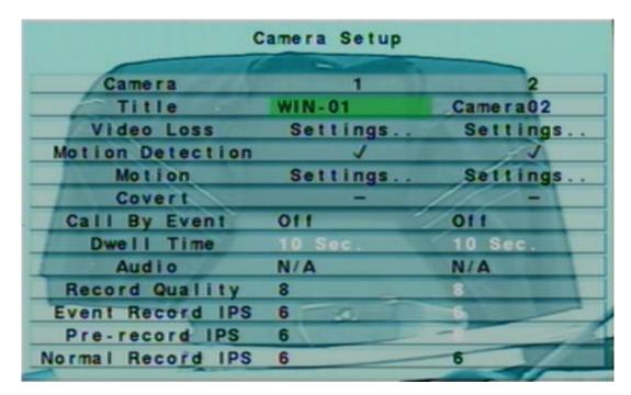
The Camera Setup allows the administrator to define the attributes for each camera. There are up to 16/9 cameras which can be connected to the system.
