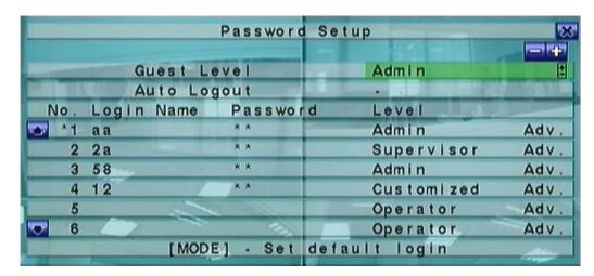
The Password Setup allows the administrator to add new users, delete existing ones, and/or modify the user's name, password, and/or level.
