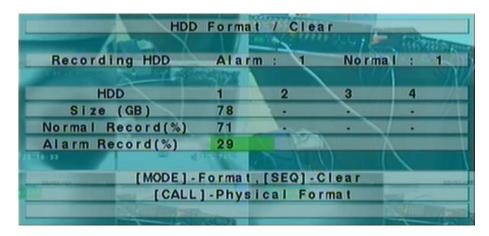
Each of the HDDs must be formatted before it can be used to record video/audio. The HDD Format/Clear screen allows the administrator to format and/or clear each HDD, and set the size for Alarm Record partition and Normal Record partition for each HDD. Please note that the HDD IDs for the internal HDDs in the DVR start from ID 1.
